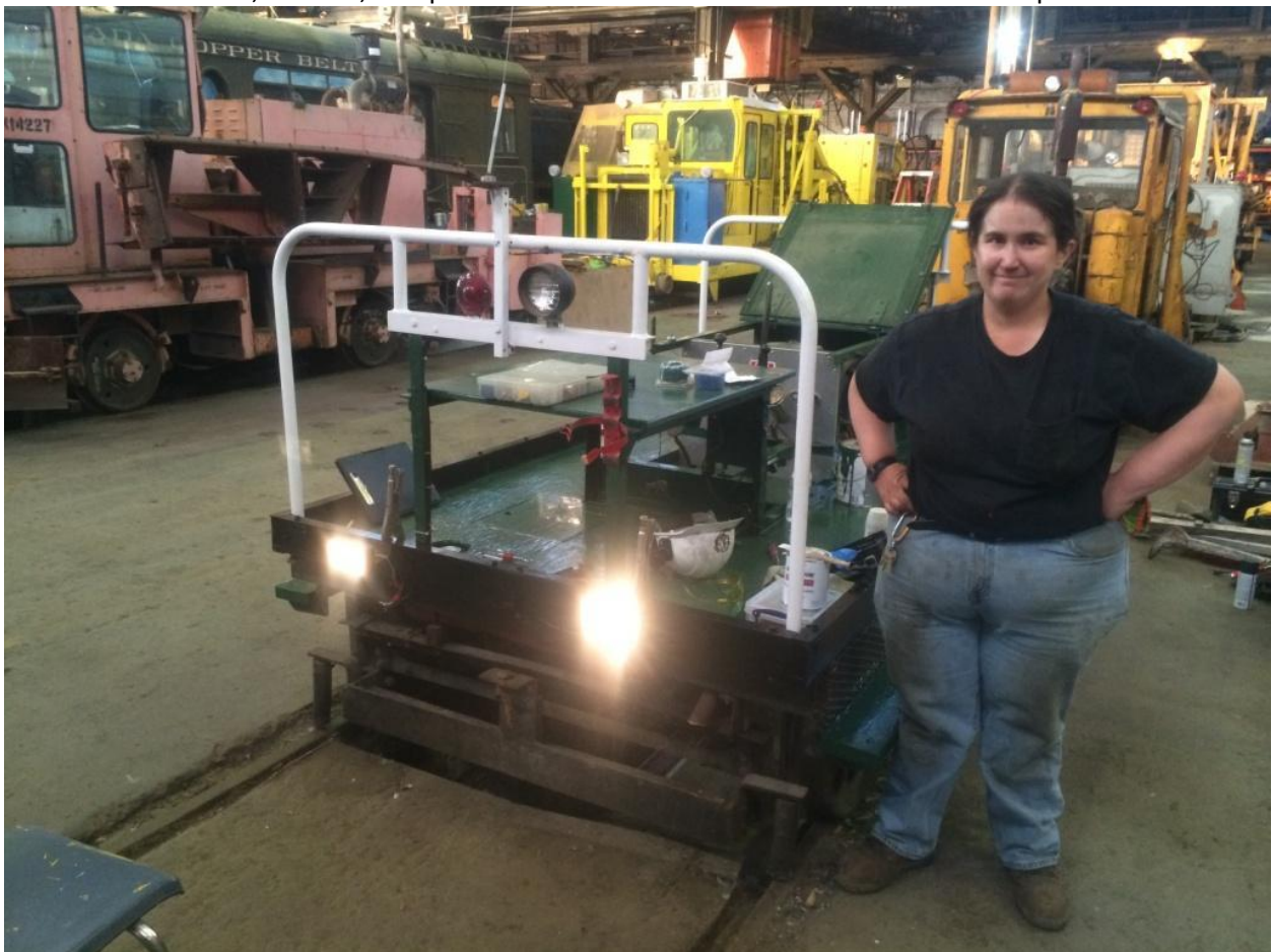
Heather after having successfully hard-wired the work-lights on the 60 A-6 motorcar, which she painted, as well.
