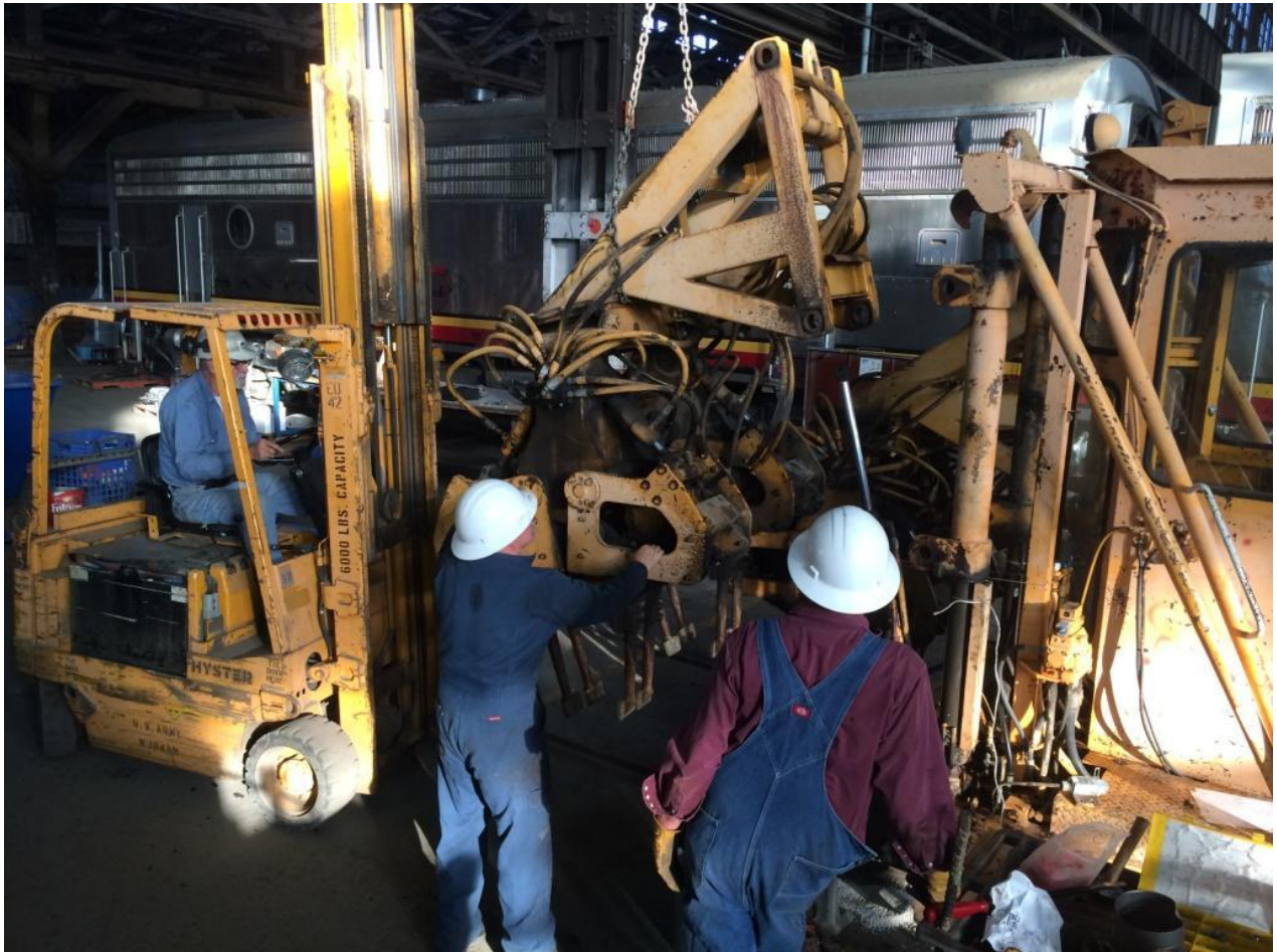
Alan, Mike H., Cliff position the second work-head on the old-old tamper
