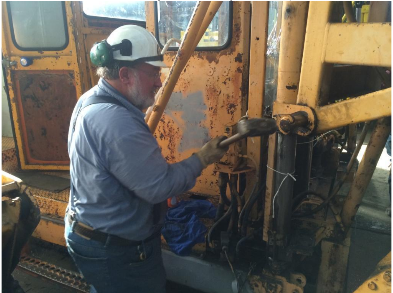
Frank swinging the 20 pound sledge driving in a pin that holds the work-head on the old-old tamper
