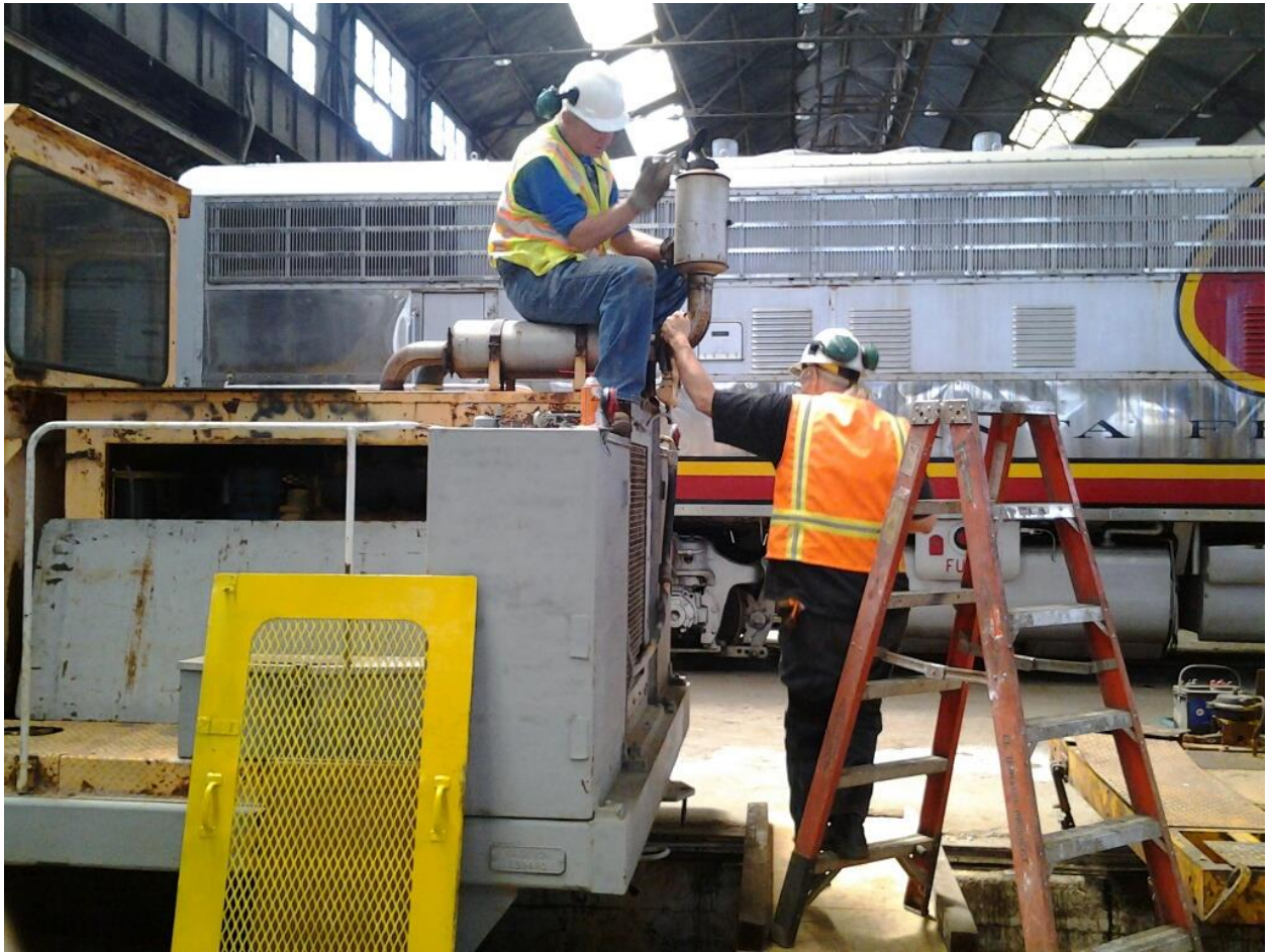
Steve and Fred transferred the spark arrester from old-old tamper to new-old tamper
